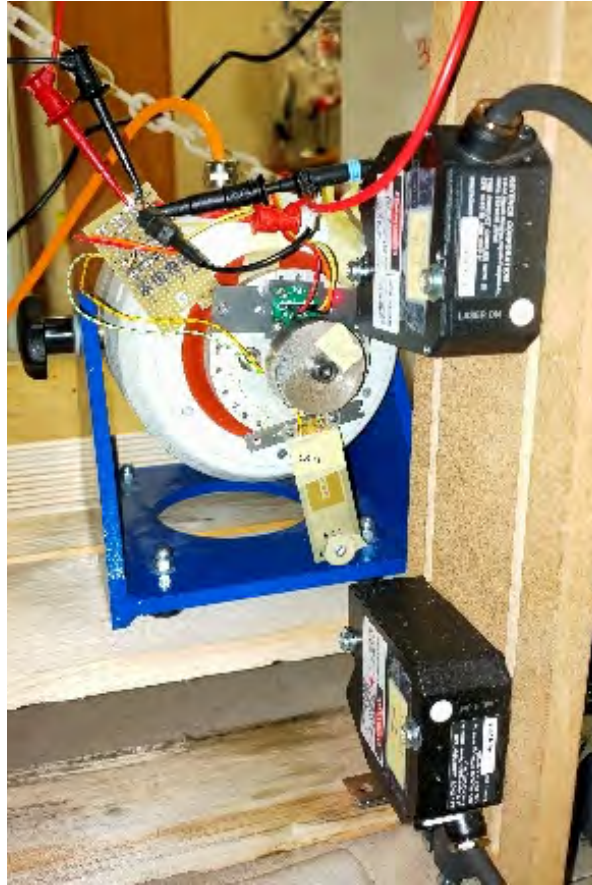
Figure 2. A picture of the experimental setup, including a view of the electrodynamic shaker, the laser distance measurement sensors, the piezoelectric transducers with the 3D printed assembly structures.
