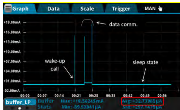
Figure 18. Power consumption of the actuator node with WuR when a wake-up call and data communication is performed (communication phase). A 32.7 \mu\text{A} average current is computed in a 60 s reference period as highlighted in red.
